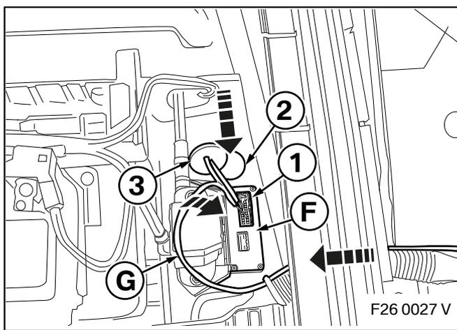
Insert the plug of tailgate silencer wiring harness **G** into the large socket (1) of tailgate silencer receiver unit **F**. Push the rest of the cable through the opening in the floor (2) and push the stops (3) into place.
