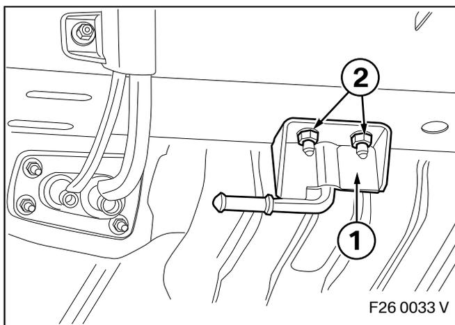
Remove the two nuts (1) from the rear silencer mounting (2).
