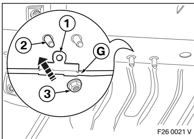
Place the fastening (1) of tailgate silencer wiring harness **G** on the stud bolts (2) and screw into place using the existing nuts (3).
