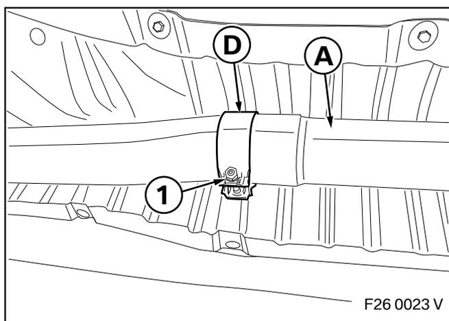
Align clamp **D** so that the screw (1) points downwards. ◀
