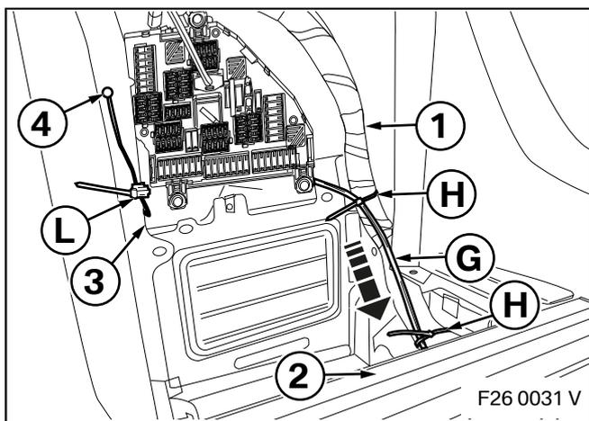
Route tailgate silencer wiring harness **G** downwards and tie it at a suitable point using cable ties **H** to the large wiring harness (1) and route this below the rail (2) into the luggage compartment.
