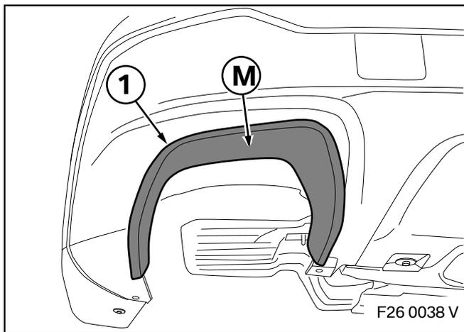
Attach finisher **M** and transfer the rear contour (1) to the rear apron using a suitable tool. Remove finisher **M**.
