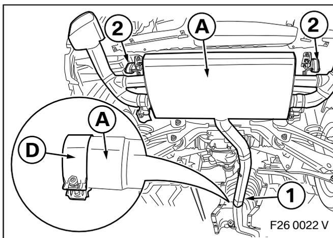
Place clamp **D** on the pipe of tailgate silencer **A**.
