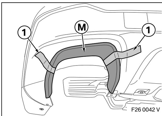
Secure finisher **M** with suitable adhesive tape (1) and do not remove for **around 24 hours**.
