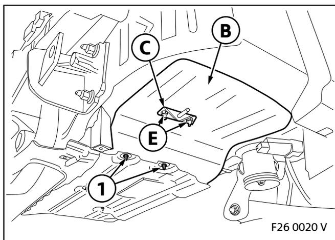
Remove the two nuts (1) from the heat insulation. Push heat insulation **B** in and re-tighten the nuts (1). Secure rear silencer holder **C** using both nuts **E**.
