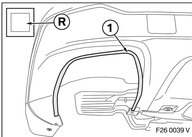
Prime the surface inside the contour (1) using primer **R**.
