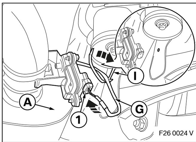
Insert the plug (1) from tailgate silencer wiring harness **G** into the socket of the tailgate switch of tailgate silencer **A**.
