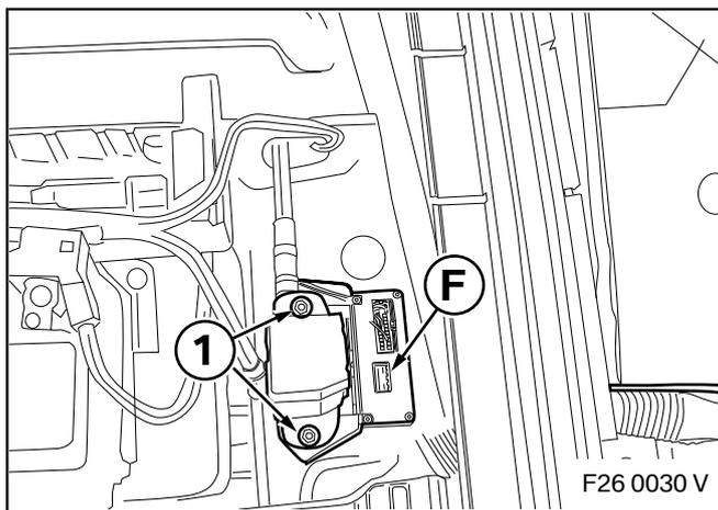
Release the two nuts (1) from the handover support point and affix tailgate silencer receiver unit **F** underneath, then secure the handover support point again using the two nuts (1).
