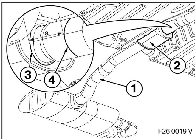
With the existing exhaust system (1), measure a length of **a = 43 mm** in front of the housing for the middle silencer (2) from the wall (3) and transfer a line (4) using suitable tools.
