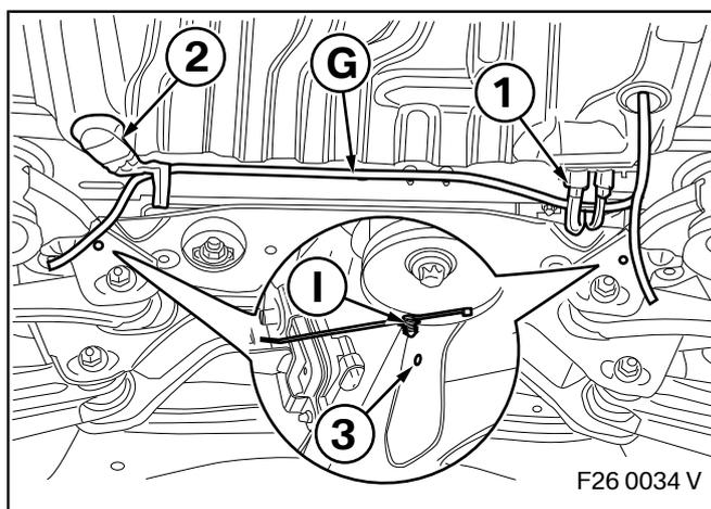
Route tailgate silencer wiring harness **G** below the cable (1) and (2) on the left-hand side and secure with cable tie **H**.
