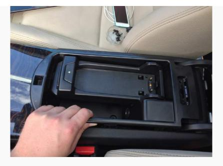
Next we need to detach the cradle from the cubby. Start by removing the T10 screw on the passenger side (in a LHD vehicle at least). Once you remove the screw, set the plastic disc aside.
