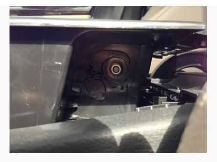
Then you should be able to pull the cradle up, you may have to unhook it one side at a time. There are little gear things that can pop out pretty easily and get lost, you can see it in the photo above with an 'R' stamped on it. One of mine fell into the abyss that is my center console, never to be seen again. Try to keep track of them if they do come out, as they're easy to snap back in.
