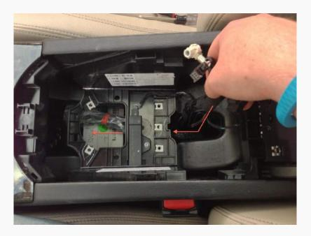
Now it's time to transfer the couple plugs from the old cubby to the new one. Obviously, this step is only necessary if you're replacing the cubby. If you aren't feel free to skip ahead to step 12.
