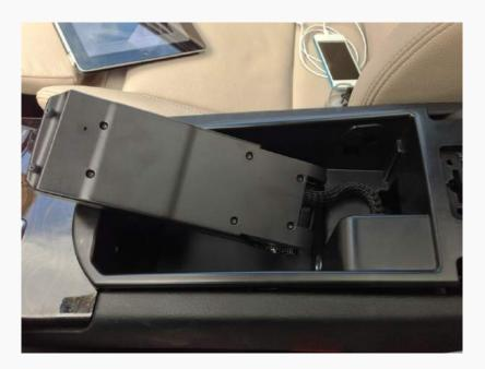
Once the screws are undone the two halves come apart easily. Push the bottom half towards the back.
