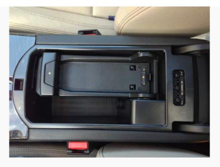
Lift up the phone cradle and pull out the rubber false bottom, it should come right up. Remove the 4 T20 screws that have been exposed.
