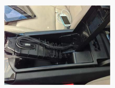
Next we need to gain access to the middle part where the electronics are. There are some tabs to push on with the small flathead. They let go pretty easily.
