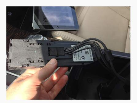
Now we need to gain access to the electronics inside this part. This portion is a little difficult, as there are a lot of small clips holding this together. Start towards the front and work your way around and back.
