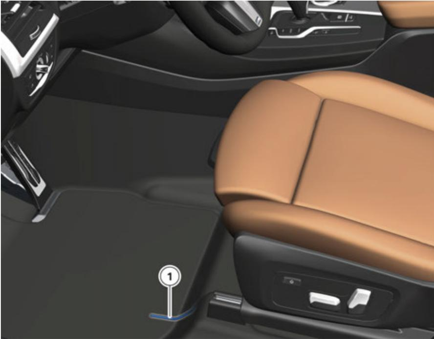
G01 Vehicle WLAN antenna
