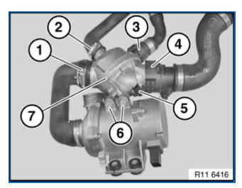
Release hose clamp (1) and detach coolant hose.
