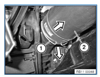
Detach pressure pipe (2) on right from charge air cooler in direction of arrow.
