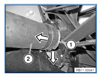
Release lock (1) with a suitable tool.
