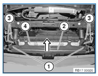
Remove expanding rivets (1).
