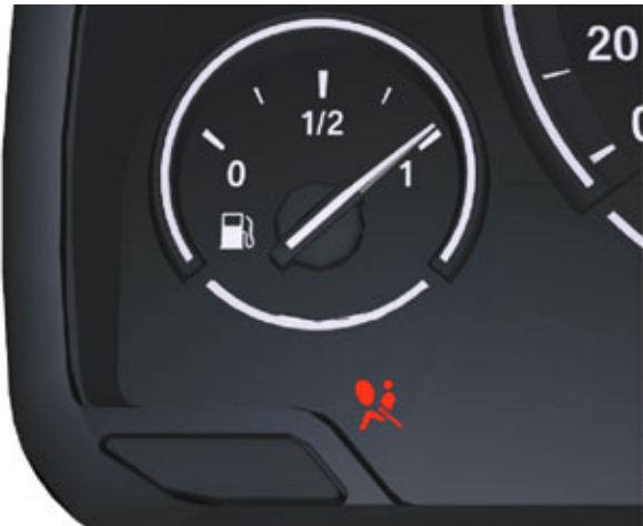
F25 Airbag indicator light (example shows high version of instrument panel)
