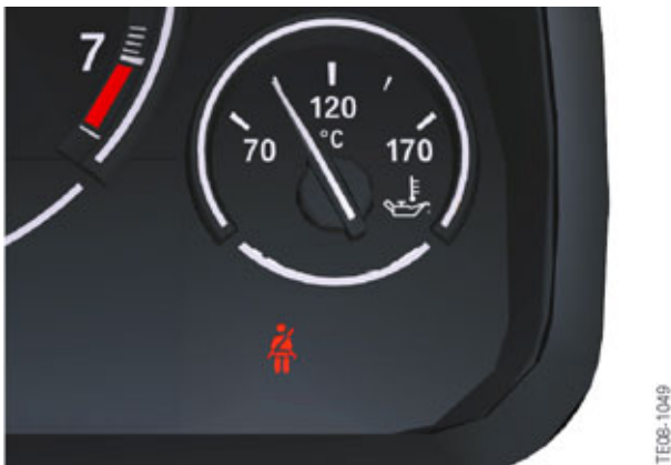
F25 Seat belt warning light (example shows high version of instrument panel)
