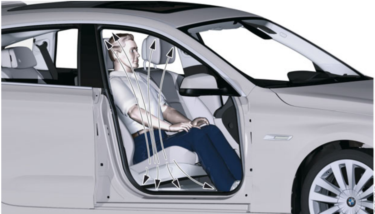
Measuring procedure of CIS mat using F07 as example
