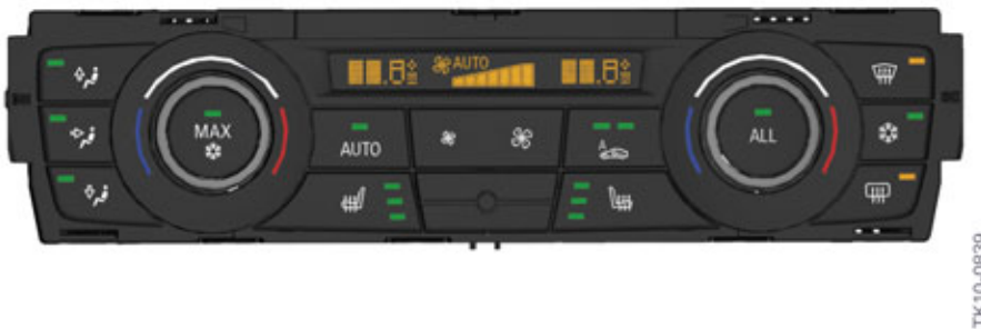
F25 Control panel of 2/1-zone IHKA
