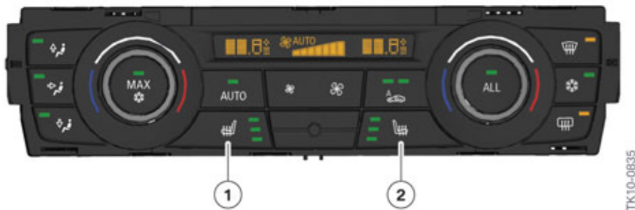
F25 IHKA control panel
