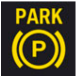
F25 Indicator light showing parking brake fault
