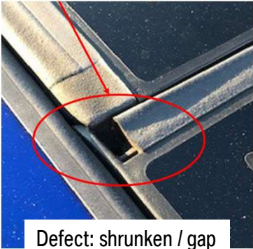
Defect: shrunken / gap
