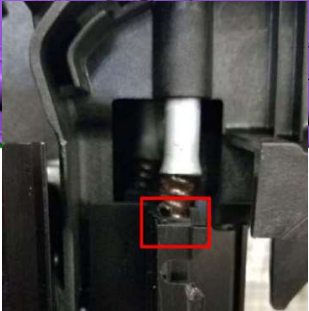
Defect: misaligned or burr
