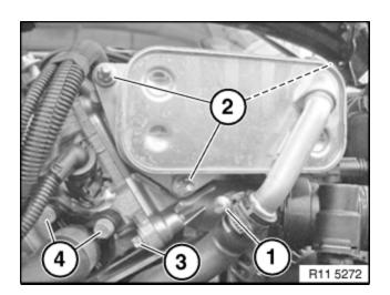
Release coolant hose (1). Tightening torque: <u>11 42 4AZ.</u> Unfasten screws (2). Tightening torque: <u>11 42 3AZ.</u> *Installation note:* Replace all gaskets. 11 44 000 Removing and installing/replacing oil-to-water heat exchanger (N52T)
