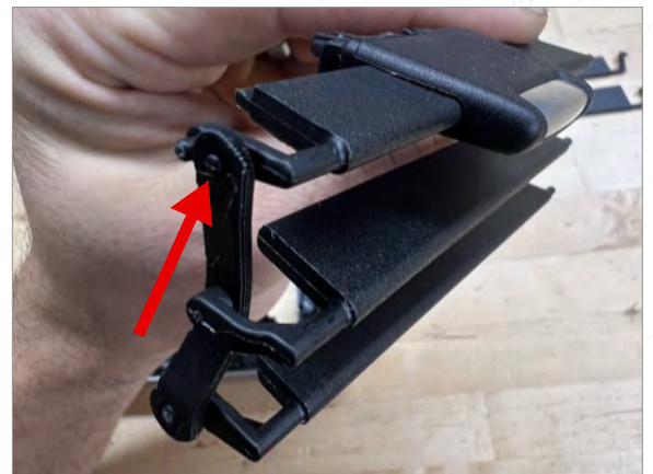
5b Assembly should look like this (use front peg on top slat)
