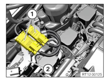
Attach connector (1) of the primary oxygen sensor and the monitoring oxygen sensor to the cable duct(2).
