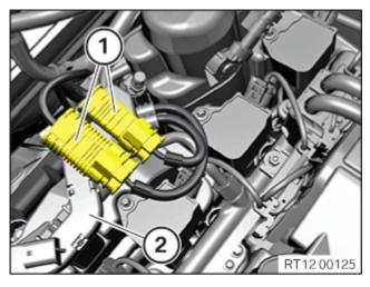
Release connector (1) of the primary oxygen sensor and the monitoring oxygen sensor from the cable duct (2) and place to one side.
