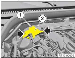
• Loosen service opening (2) in marked areas (arrows) and turn to one side via the pivot point (1).
