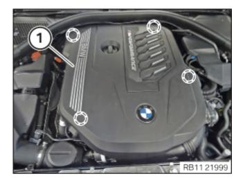
Release the acoustic cover (1) upwards out of the rubber mounts (markings).
