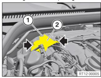
Maneuver sound insulation (2) over pivot point (1) into installation position and maneuver into marked areas (arrows).
