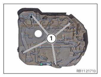
• Check that rubber mount (1) fits correctly in acoustic cover.
