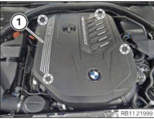
• Install acoustic cover (1) and attach it in the rubber mounts (marks).
