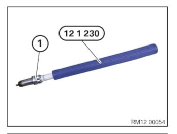
Insert spark plug (1) in the special tool 0 496 065 (12 1 230).
