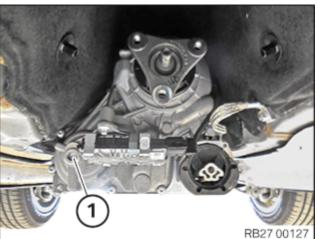
Top up the transmission oil with the special tool 0 493 337 (00 2 080) up to the lower edge of the opening for the oil filler plug.
