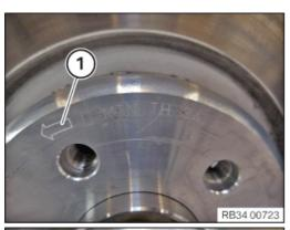
If an arrow 1 is stamped on the brake disc, it must point in the direction of travel.
