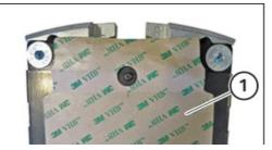
Pull off the protective film of the adhesive layer (1) at the brake pads.
