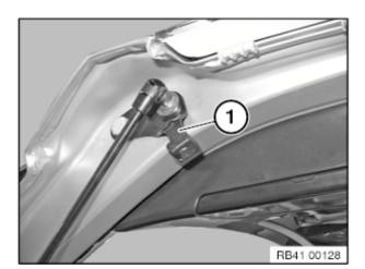
Check holder (1) left and right for damage, replace if necessary.
