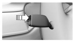
Continue to press the button on the turn signal lever until the desired widget is selected.
