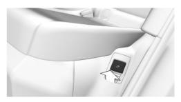
Pull the lever and apply your weight to the rear seat backrest or lift it off, as necessary.
