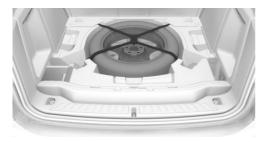
The emergency wheel and the wheel change tools are located in the cargo area under the cargo floor panel.
