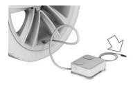
With standby or drive readiness turned on, turn on the compressor and let it run for a maximum of 10 minutes. When the tire pressure does not reach at least 2 bar, contact a manufacturer service center or another qualified service center or repair shop.
