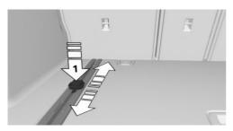
To slide the lashing eyes, press the button, arrow 1. Make sure that the lashing eyes latch at the new position.
