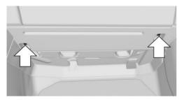
Loosen fasteners, arrows, and open cover.
