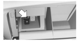
Insert the fragrance cartridge without pressure into the cartridge holder. The cartridge snaps lightly into place.
