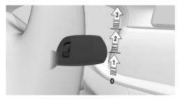
Activate: press the lever up once from its 0 position, arrow 1.
