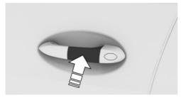
Hold activated Key Card directly and centered on the external door handle of the driver's door.
