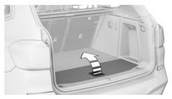
2. Lift the cargo area floor up until it is over the multifunction hook.
