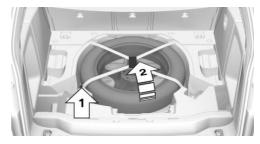
5. Remove the emergency wheel from the storage well, arrow 2.
