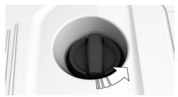
Only add engine oil when the message is displayed in the instrument cluster.
