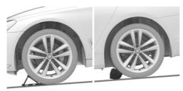
If you need to change a wheel on a slight downhill grade, place chocks and other suitable objects, for instance rocks, under the wheels of both the front and rear axles against the rolling direction.
