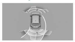
The approach of the vehicle to an object is shown on the Control Display. Objects that are farther away are already displayed on the Control Display before a signal sounds.
