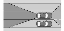
Radar sensors monitor the space next to the vehicle when traveling faster than a minimum speed of up to approx. 130 mph/210 km/h.
