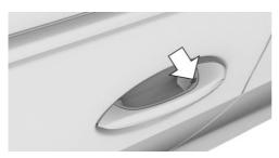
Touch the grooved surface on the handle of a closed vehicle door with your finger for approx. 1 second without grasping the door handle.
