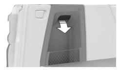
2. Open the bracket and take the warning triangle out in the direction of the car's interior.
