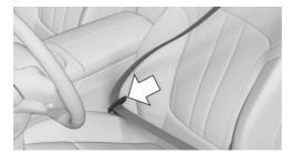
To ease accessibility to the safety belt buckle, an adjustable slider is available on the belt to help position the buckle when not in use.
