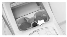
A socket is located between the cup holders. Pull off the cover.
