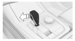
Press the selector lever to the left from selector lever position D.
