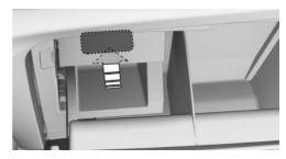
Remove the cover of the fragrance cartridge. Hold the cover on the top to slide it from the fragrance cartridge.
