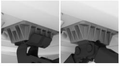
3. Extend the vehicle jack by turning the vehicle jack crank or lever clockwise.
