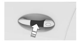
Hold the near field communication antenna of the smartphone directly and centered on the external door handle of the driver's door. The position of the near field communication antenna depends on the smartphone model.
