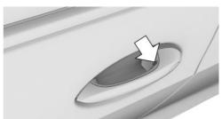
Touch the grooved surface on the handle of a closed vehicle door with your finger and hold it there without grasping the door handle.
