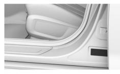
The vehicle identification number can be found on the nameplate, on the left-hand side of the vehicle.
