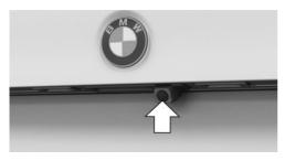
The camera is located in the handle of the tailgate.
