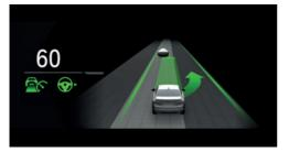
Example: the indicator/warning lights for the Active Cruise Control with Stop & Go function ACC and the Lane Change Assistant indicate a lane change to the next lane. At the same time, the lane change to the next lane is shown with animation in the Assisted Driving View.
