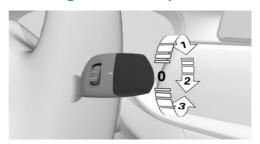
Turn the outer switch upward.
