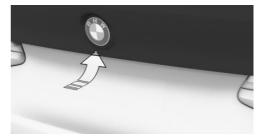
▶ Unlock the vehicle and then press the button on the outer side of the tailgate.
