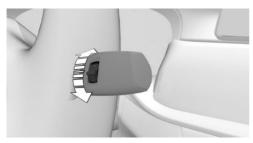
Turn the thumbwheel on the wiper lever.
