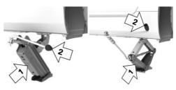
Insert the vehicle jack into the rectangular recess of the jacking point closest to the wheel to be changed.
