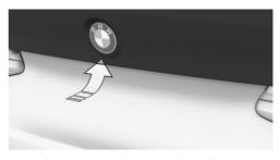
Press the button on the outer side of the tailgate.
