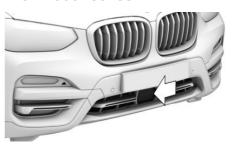
The radar sensor is located in the front bumper.
