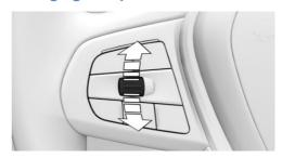
Press the rocker switch up or down repeatedly until the desired speed is set.
