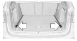
To secure the cargo there are additional movable lashing eyes in the cargo area.
