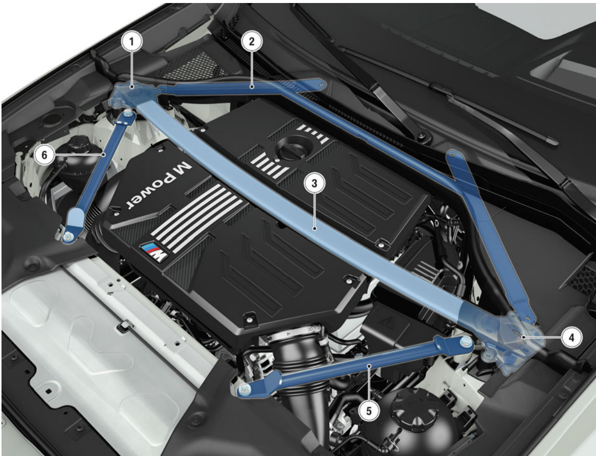
F97/F98, stiffening measures in the forward area
