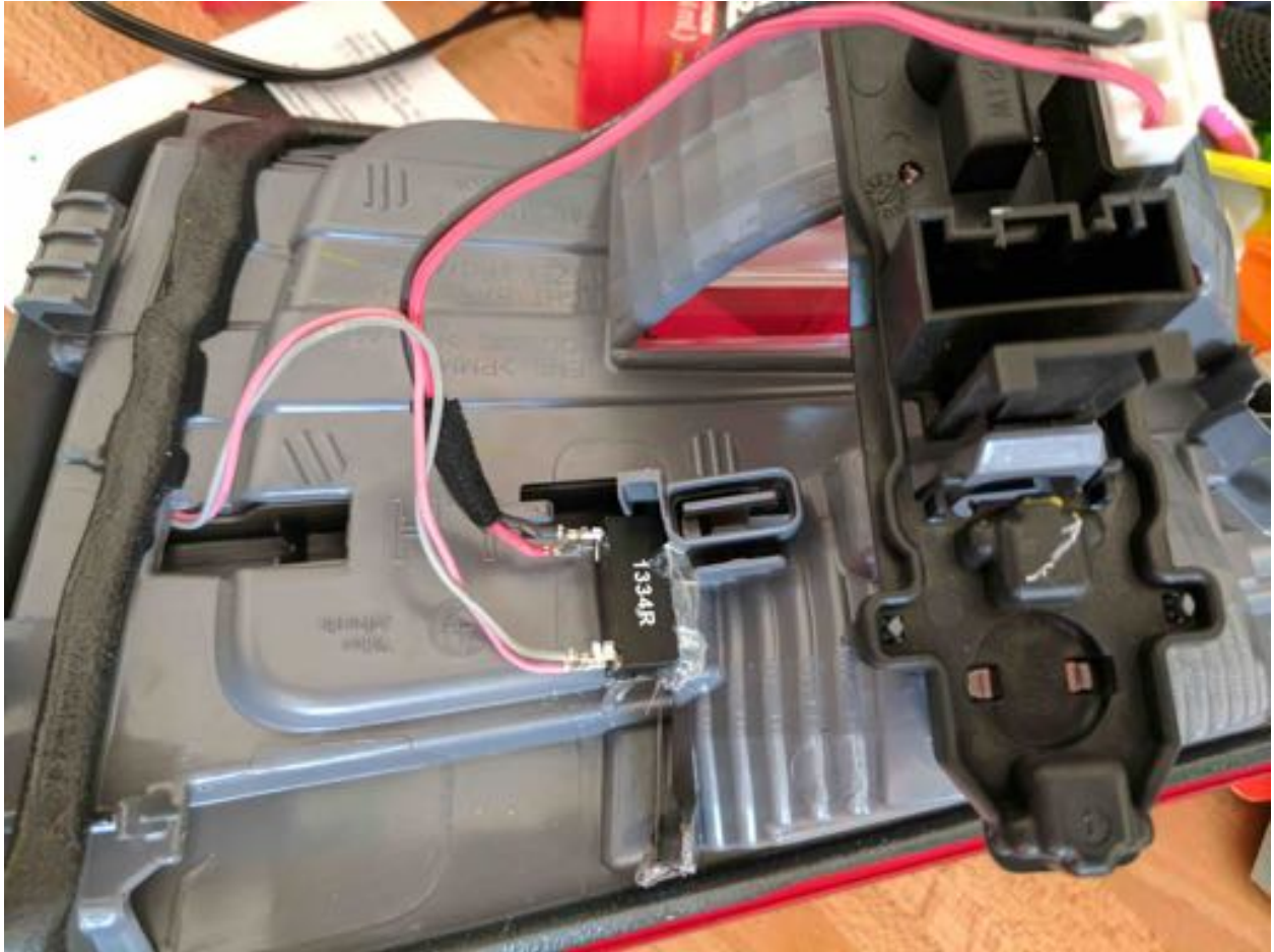
Fig 04 Hot glue the LDD-500L module into place where the Valeo board used to be. You are all done!
