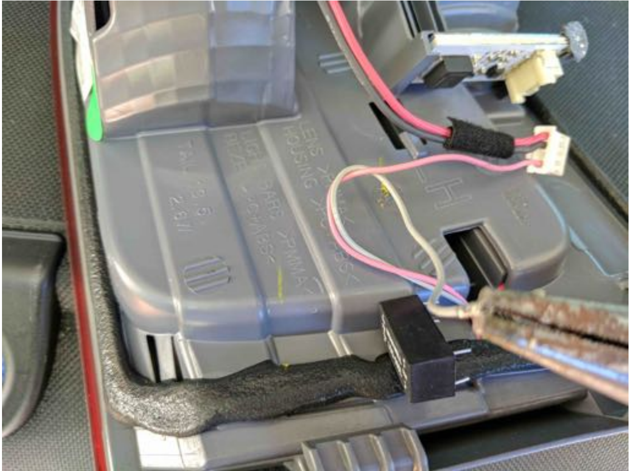
Fig 02 Crimp the plug a little bit so you have a snug fit onto the pin of the LDD module.
