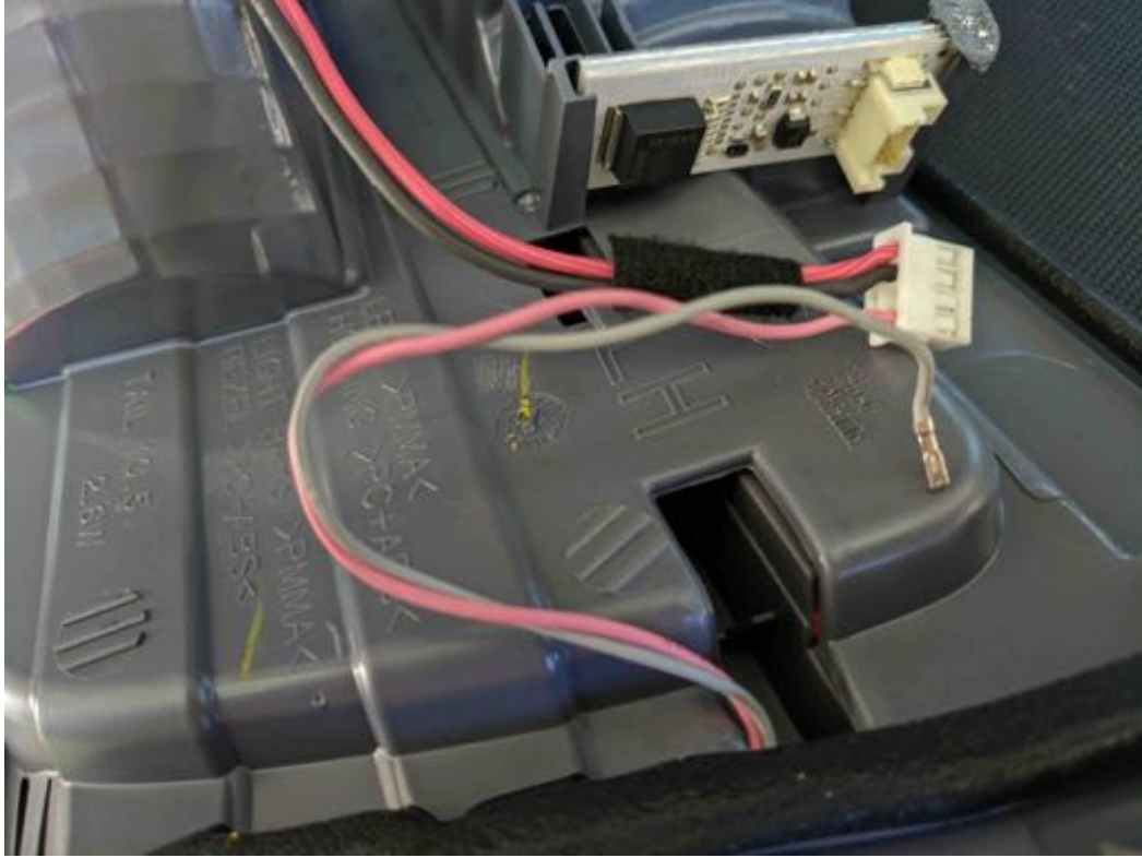
Fig 01 Gray wire Plug removed from Harness
