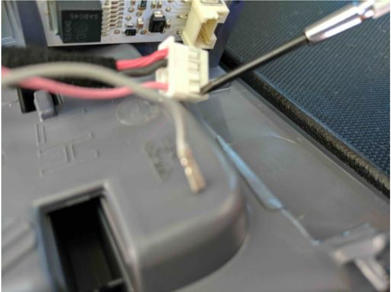
Fig 00 Remove the plug from harness by inserting a safety pin or jewelers screw driver under white tab and gently lifting while pulling on wire.
