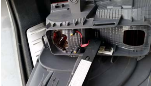
Small pry bar used to lever circuit board loose on fender light assy. Tailgate assembly requires heat stake to be broken for board removal.
