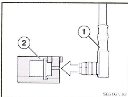
2. Disconnect the violet connector on the shark fin antenna and remove the violet housing (2) from the coax cable (1). Note: Unlock the locking tab first when removing the housing.
