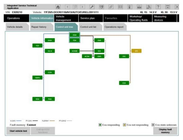
Here you can observe the ongoing determination of the control units that are fitted. If no control unit tree is available, the "Control unit list" mask is displayed automatically.
