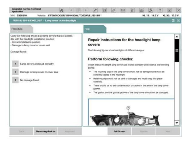
After the test plan has been completed, you should carry out the "Delete fault memory" function.
