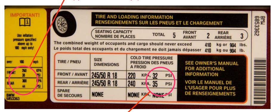
Front Pressure 32 psi Rear Pressure 35 psi (speeds below 100 mph)
