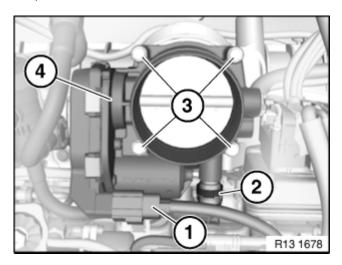
Release connector (1) and remove.
