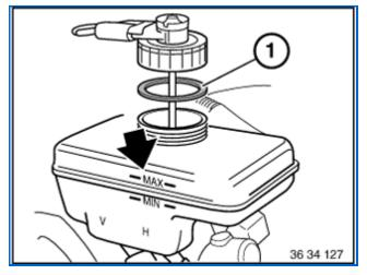
Switch off bleeder unit and remove from expansion tank.
