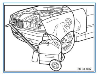
Connect brake fluid changer to expansion tank and switch on.
