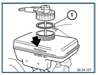
Switch off brake fluid changer and remove from expansion tank.
