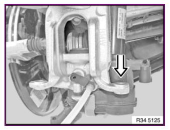
Disconnect plug connection on EMF actuator and detach cable from cable clip.
