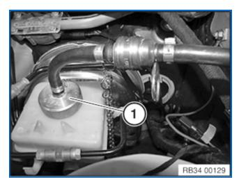
Connect bleeder unit to expansion tank and switch on.
