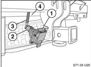
Secure trailer wiring harness (2) to vehicle plastic bumper guide with wire-tie clip assembly (1) as illustrated.
