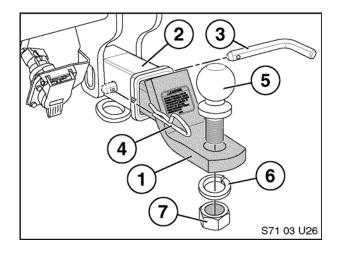
Install trailer ball (5) to ball mount (1) with lock washer (6) and nut (7).
