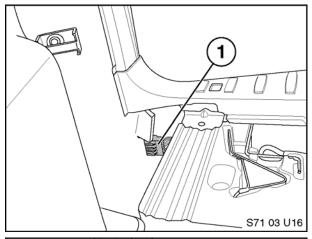
1. Locate vehicle connector (1) in right side storage well area.
