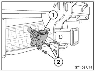
Install 7-pin trailer connector (1) onto mounting plate as illustrated with four T25 TORX® head screws (2) from installation kit.
