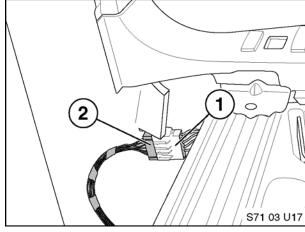
Plug trailer hitch wiring harness connector (2) into vehicle connector (1) and route excess harness cable behind sound insulation material.
