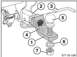
2. Install trailer ball (5) to ball mount (1) with lock washer (6) and nut (7).
