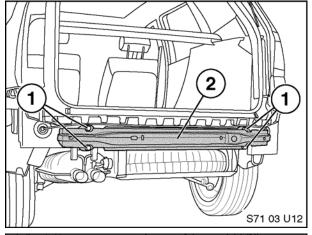
1. Remove and discard the four mounting nuts (1) and steel bumper (2) from vehicle.
