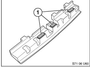
3. Attach double sided adhesive tape to bumper insert. **P/N 51 12 3 416 322.**
