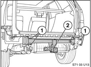
Install trailer hitch (2) using four new nuts(1) from installation kit.
