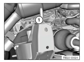
Release screws (1). Remove engine support arm. Tightening torque <u>22 11 3AZ</u>.
