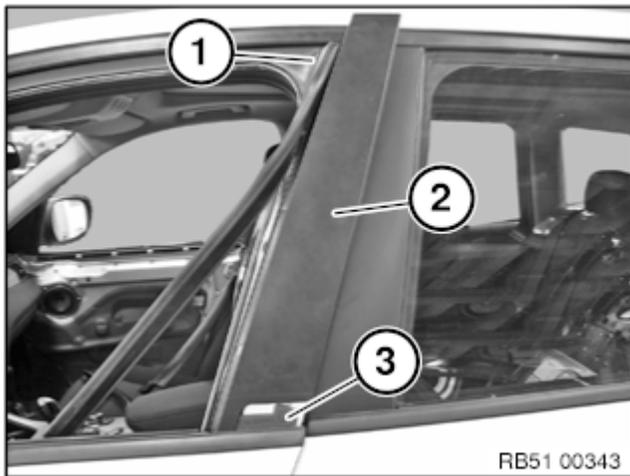
Push trim cover on window frame (2) down slightly until it can be fed out at the top at the rubber window seal (1).
