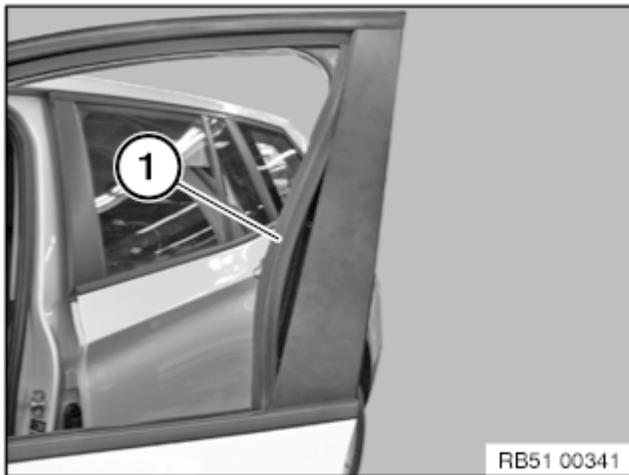
Pull rubber window seal (1) out of rear window guide. *Installation note:* Moisten rubber window seal (1) slightly with water to facilitate installation.
